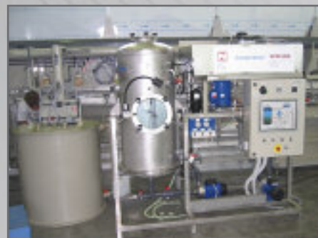
Vacuum evaporator for avoidance of waste water
