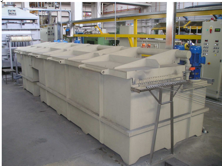
General view of a Sirio Wire ultrasonic cleaning line
