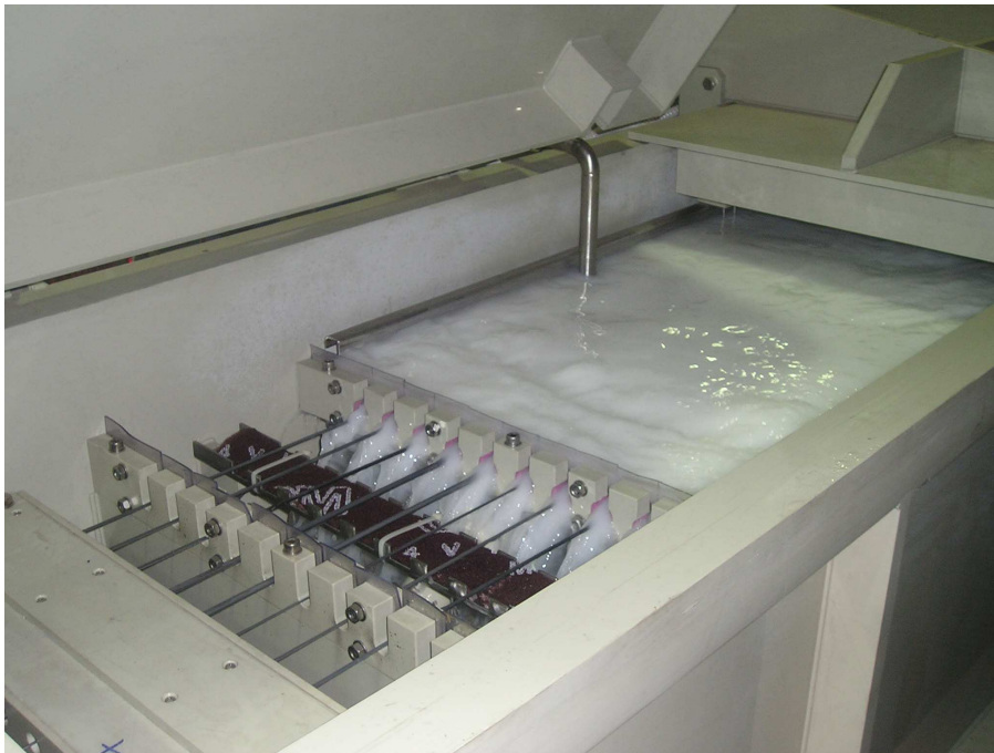
View of an ultrasonic cleaning bath, drop trap and air wiping
