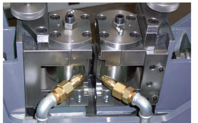
Edger rolls, either driven or non-driven, according to the process request.
