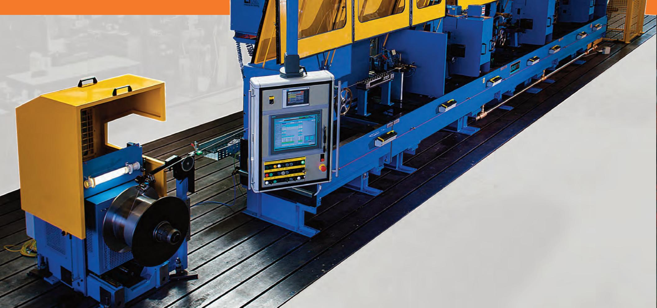
Duo Roll set with carbide rolls and bearing lubrication by means of oil circulation.
