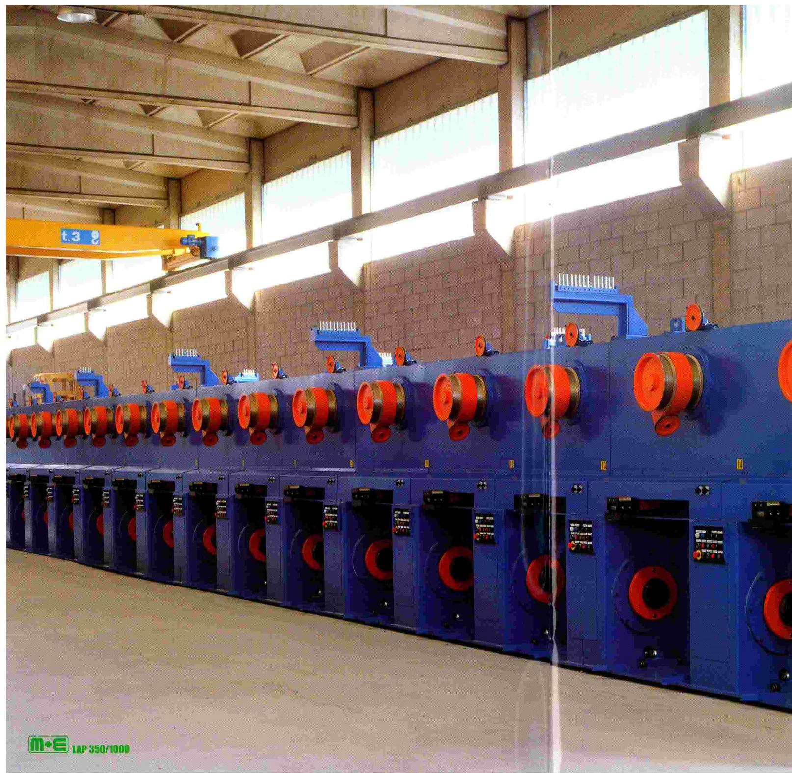
The accumulation capstans are typically used to pay-off and take-up, on spools, annealed and galvanized low carbon wire, patented and phosphated or galvanized high carbon wire, hard drawn and galvanized high carbon wire (ACSR), patented and brass coated high carbon wire (Steel Cord), hard drawn and bronze coated high carbon wire (Bead Wire), aluminum-cladded high carbon wire.
