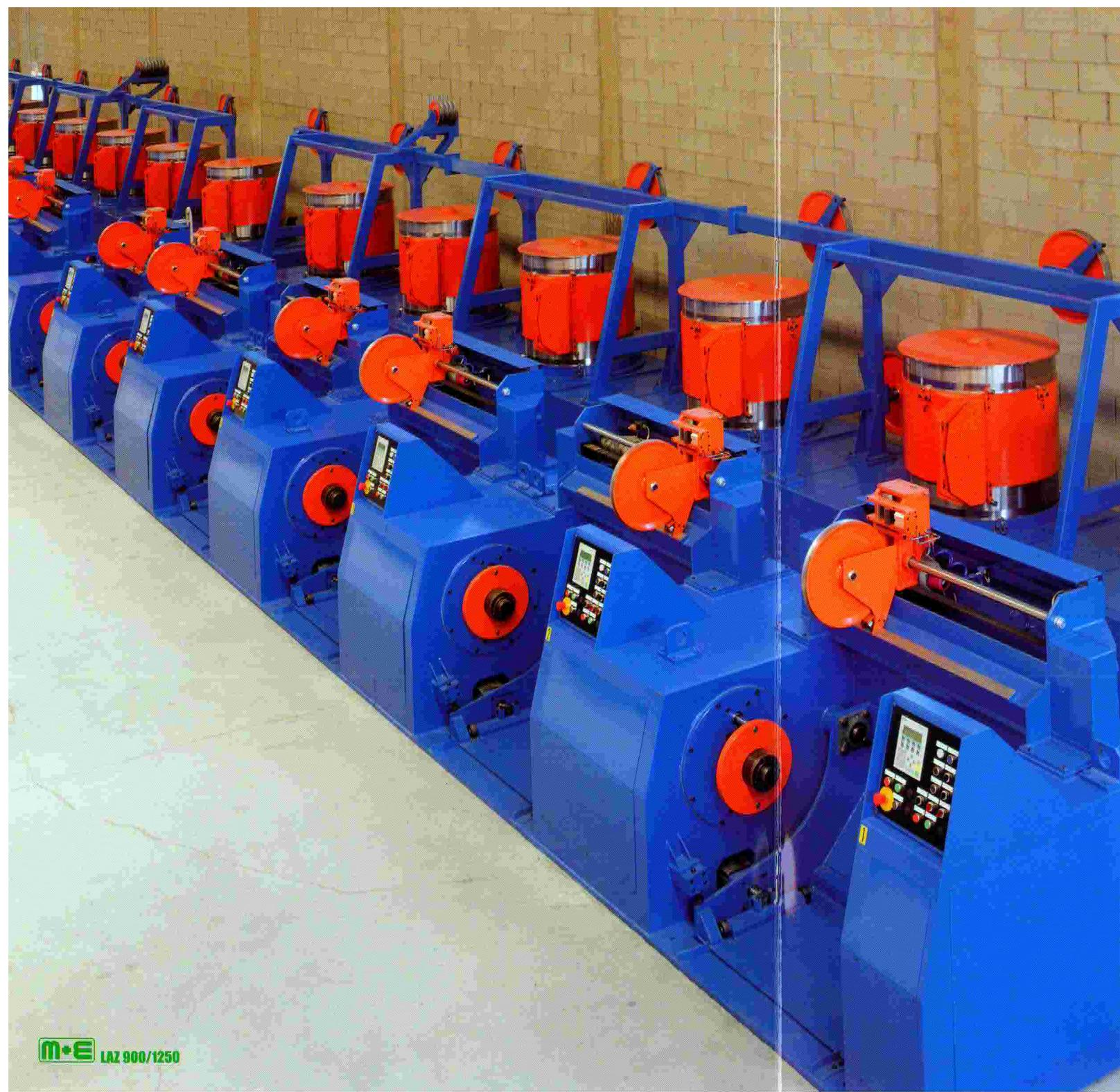
The machine frame consists of heavy duty fabricated steel segments, each providing a mounting for two or more spools.
