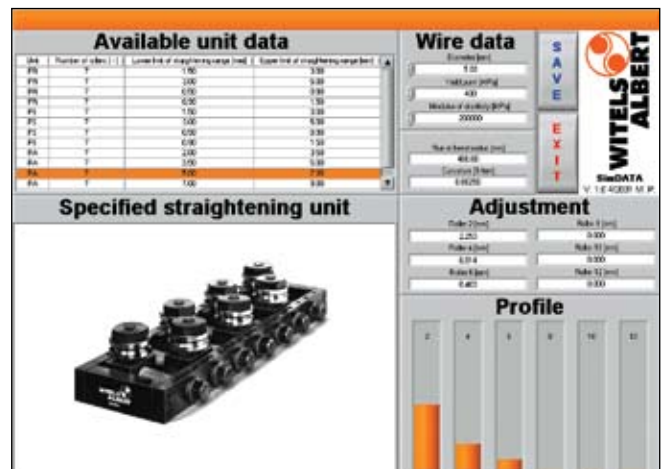
Figure 6: SimDATA software determines roll-adjustment values.
