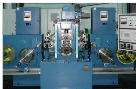
Typical BÜHLER REDEX Strip Rolling Mill configuration (i.e. equipped as a high precision equipment for noble metals processing).
