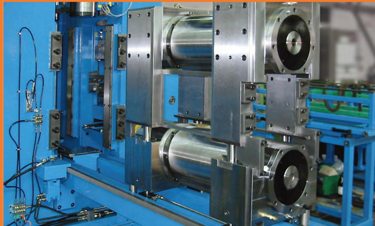
Winding unit featuring strip tension measurement and closed loop control.
