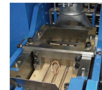
Scrapper unit in a cladding rolling mill
