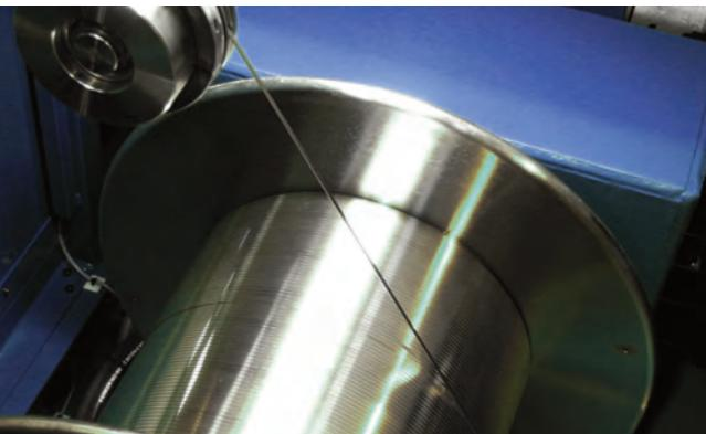
Traversing spooler with advanced feature for precise layer winding
